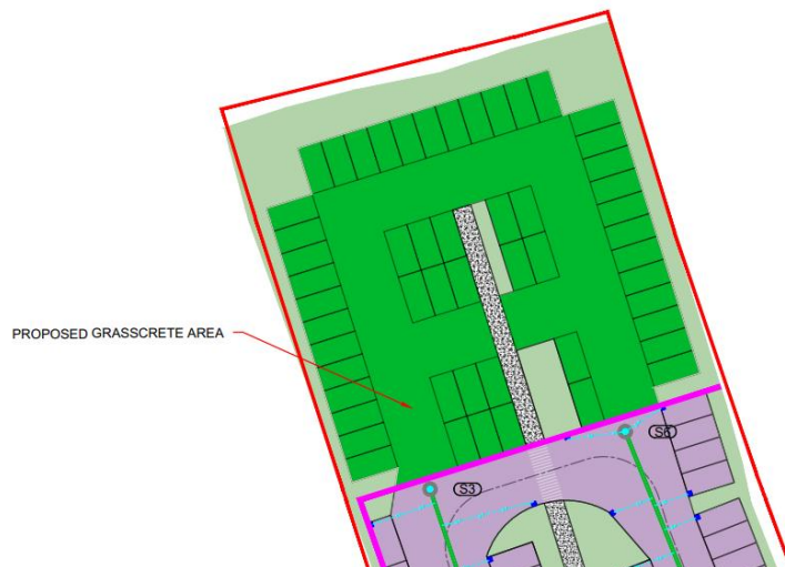
Figure 5-1: Drawing Showing Proposed Grasscrete Paving in Overflow Car-Park
